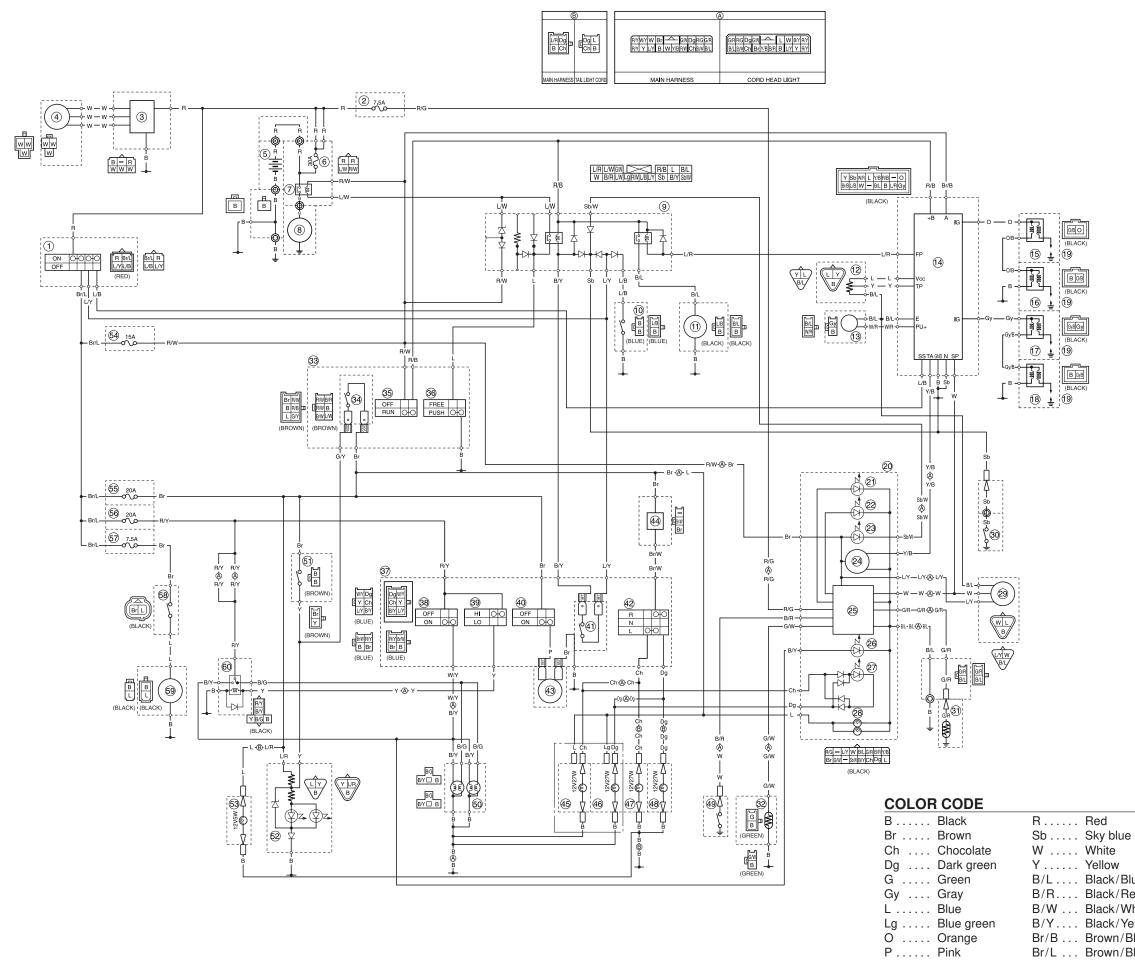
(1) Main switch (2) Fuse (back up) 3 Rectifier/Regulator (4) A.C. magneto (5) Battery (6) Fuse (main) 7 Starter relay (8) Starter motor (9) Starting circuit cut-off relay (10) Sidestand switch (11) Fuel pump 12 Throttle position sensor
